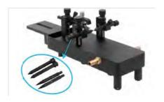
This unique stereotaxic adaptor is upgraded with water cycled heating platform to use with warm water recirculator. The temperature of the platform surface is stable, uniform and comforatble. Warm water recirculator should be purchased separately.
