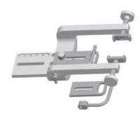
This adaptor holds the rabbits head through a dedicated cheekbone clamp, nose clip and an adjustable incisors buckle. The distance between the two cheekbone clamps can be precisely adjusted by a screw knob. An infant and an adult buckle is included. The adjustable range for the adult incisor buckle is 43,5mm, and the range for the infant one is 26,5mm. The horizontal range for the adaptor plate is 40mm.
