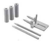
This adaptor includes earbars and raising block (65mm). It holds the head through ear canal and eye socket. The adaptor can be used with standard stereotaxic instruments or large animal stereotaxic instruments.
