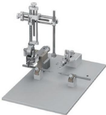
This includes a rail instead of a traditional U- frame assembly; the lateral range is wider than that of the U- frame. More manipulators can be added to this stereotax according to the experimental requirements.
